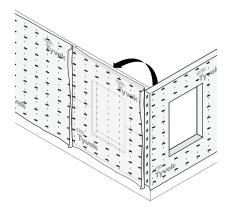
**STEP 4** Fasten the side flaps and secure the bottom flap to the foundation. For maximum air leakage reduction (when installing as an air barrier), seal wrap at the bottom of the wall with caulk, DuPont™ Tyvek® Tape or DuPont™ StraightFlash™.
