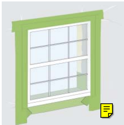
At head condition Window Flashing Tape should overlap both verticals in a shingle like manner.
