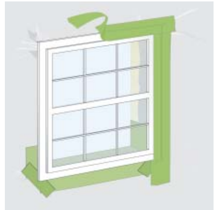
Install flanged window and apply Window Flashing Tape to both jambs (verticals) and then apply head Flashing Tape.
