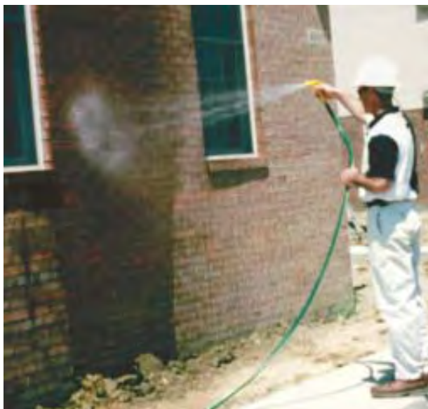
Figure 1. In this hose test, water penetrated brick veneer in less than a minute (below). The wall behind brick veneer must be designed to drain.
