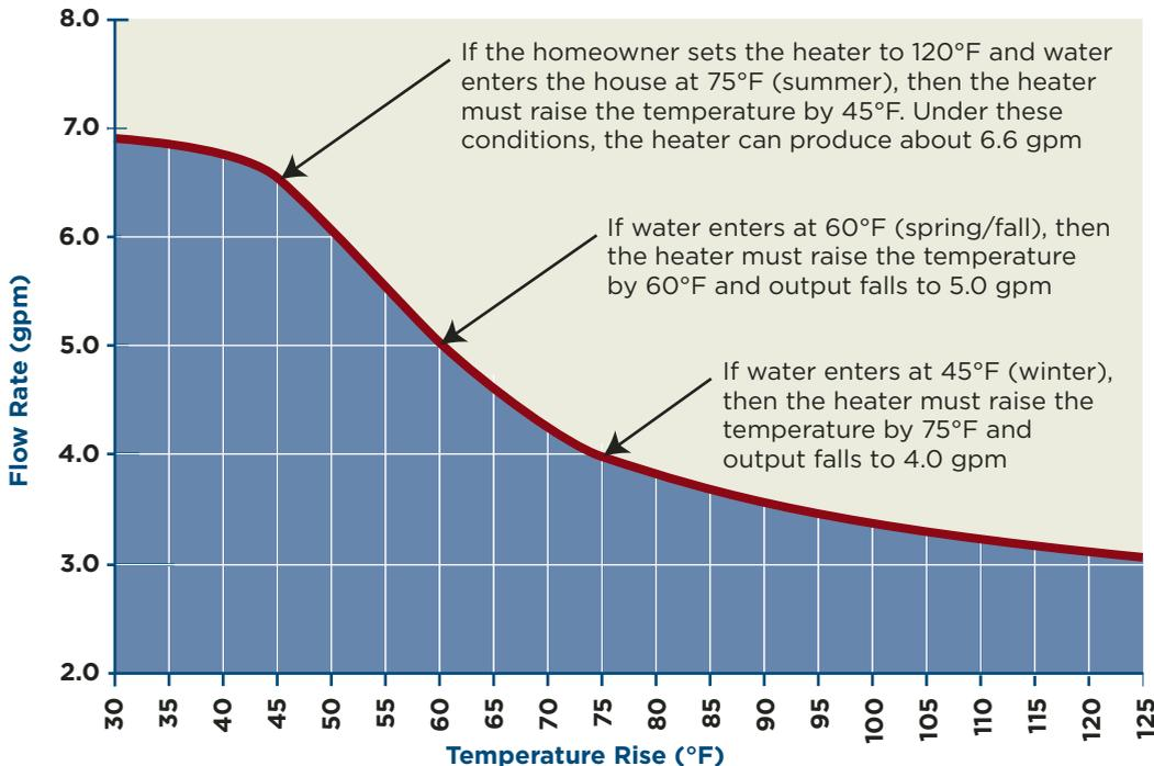
**Figure 3.** The manufacturer's specs typically include a graph showing how much hot water the unit can deliver based on input temperature, output temperature, and flow rate. This graph is typical of 185,000-Btu gas models.
