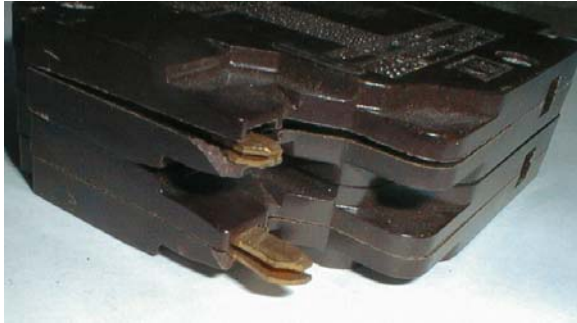
Figure 8 – Damaged “E” type breaker
